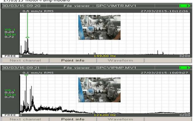
No high vibration detected, value vibration 0.5 & 0.1mm/sec No indicated misalignment detected.
